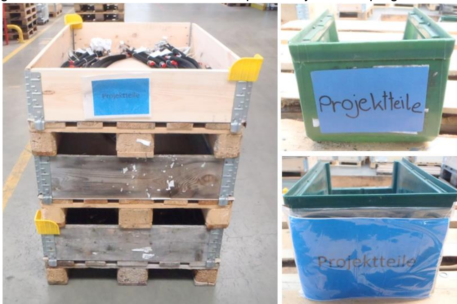
Figure 2: Sample application of the "project parts" marking on the pallet incl. stacking frame and slc
